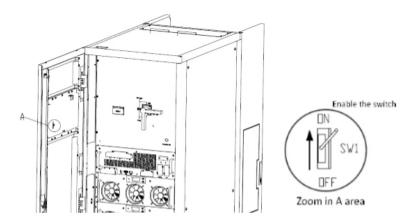
Figure 4-2 enabling the switch
