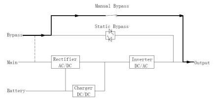
Figure 1-8 Maintenance mode operation diagram
