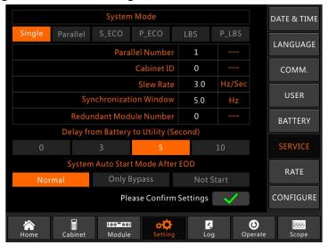
Figure 3-17 the setting interface of SERVICE
