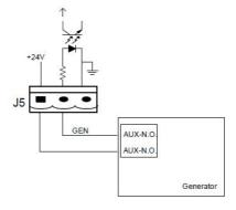
Figure 2-25 Diagram of input port for generator input Table 2-10 Description of input port for generator input
