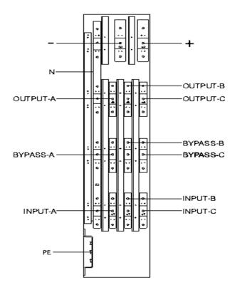
Figure 2-20 8-slot cabinet UPS connection terminals
