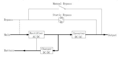
Figure 1-5 Normal mode operation diagram
