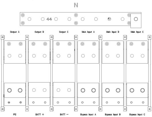
Figure 2-19 6-slot cabinet UPS connection terminals (Single input is standard, separate bypass is optional)
