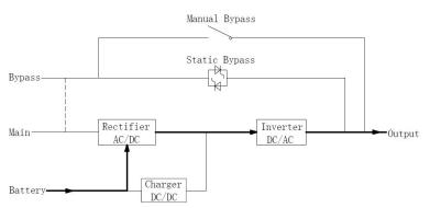
Figure 1-6 Battery Mode operation diagram
