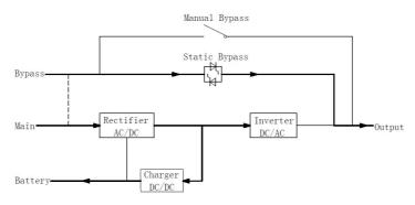
Figure 1-9 ECO Mode operation diagram
