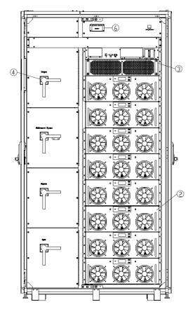
① Panel with color screen; ② Power module; ③ Bypass & monitoring module; ④ Manual bypass breaker; ⑤ Connection terminals; ⑥ SPD (optional)
