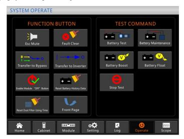
Figure 4-3 Battery maintenance
