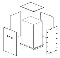
Figure 2-3 disassemble the case
