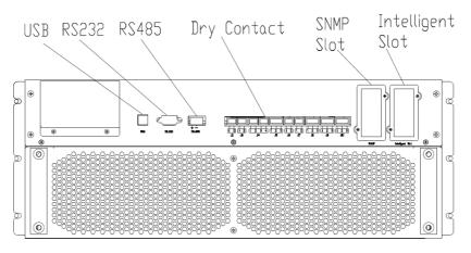
(c) Dry contact & communication interface for 8-slot cabinet UPS
