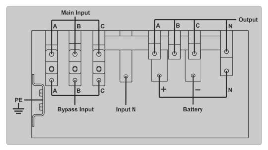
Figure 2-18 4-slot cabinet UPS connection terminals
