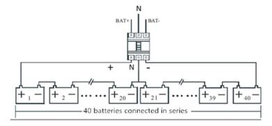
Figure 2-10 Battery string wiring diagram
