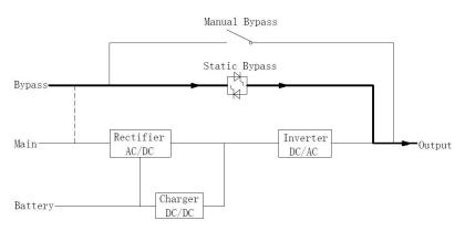
Figure 1-7 Bypass mode operation diagram
