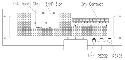
(d) Dry contact & communication interface for 10-slot cabinet UPS Figure 2-22 Dry contact & communication interface
