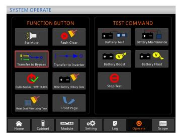
The operation interface for transferring to bypass
