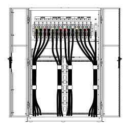
Figure 2-16 Cable Entry for 10-slot cabinet (Bottom Entry)
