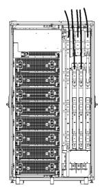
Figure 2-13 Cable Entry for 8-slot cabinet
