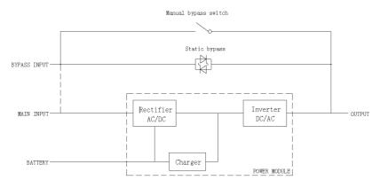
(b) 4-slot and 6-slot UPS Block Diagram
