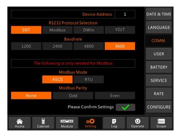
Figure 3-13 the setting interface of COMMUNICATION
