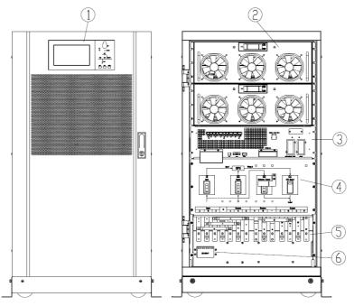
① Panel with color screen; ② Power module; ③ Bypass & monitoring unit (no hot-swappable function); ④ Breakers (input/bypass input/maintenance bypass/output); ⑤ Connection terminals; ⑥ SPD (optional)
