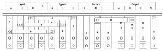
Figure 2-17 2-slot cabinet UPS connection terminals
