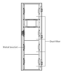
Figure 5-1 dust filters on the back side of the front door www.lbspower.com
