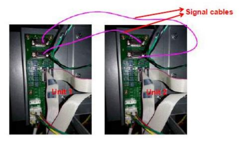
The signal cable connection for 2 UPSs in parallel b) When 3 UPSs in parallel, please operate as below.
