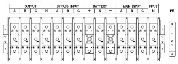
Figure 2-21 10-slot cabinet UPS connection terminals
