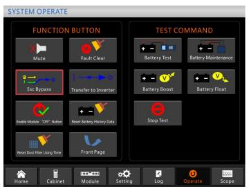
The operation interface for escaping bypass
