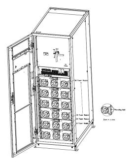
Figure 2-9 Installing power modules
