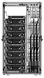
Figure 2-14 Cable Entry for 8-slot cabinet
