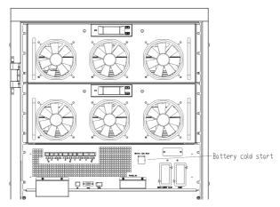
(a) Battery cold start button location for 2-slot cabinet UPS www.lbspower.com
