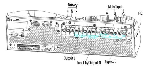
Fig. 2-16 3-phase in and 1 phase out, common input
