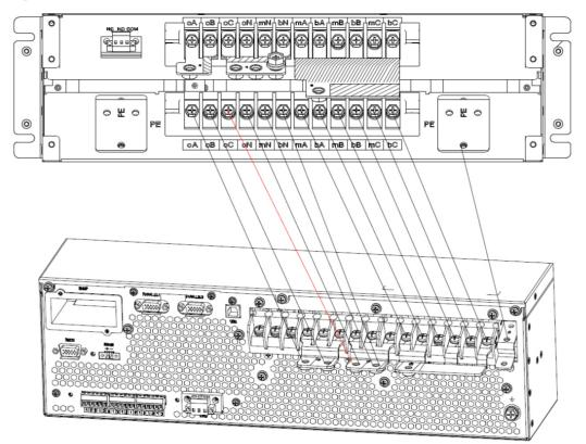
(4) 3-phase input and 1 phase output with dual input
