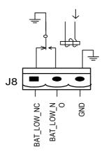
Figure 2-15 Battery warning dry contact interface diagram
