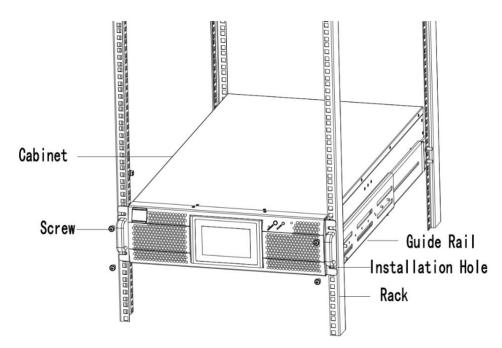
Fig.2-3 Rack Mounted Installation
