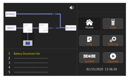
Figure 4-3 Inverter starting
