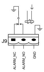
Figure 2-16 Integrated warning dry contact interface diagram Table 2-11 General alarm dry contact interface description
