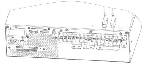
Fig. 2-17 Fix insulation film
