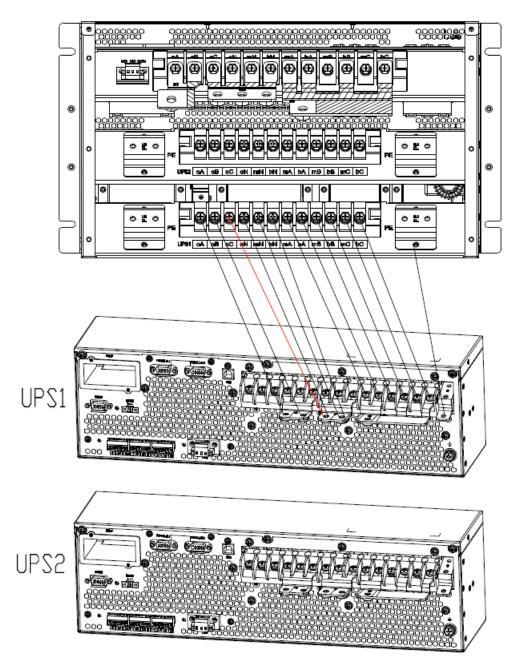
(b) 3-phase input and 1 phase output with dual input
