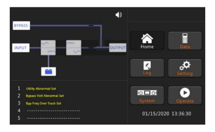
Figure 4-7 Energy flowing diagram of discharge
