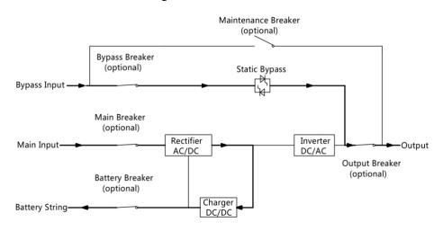
Figure 1-6 Bypass mode operation diagram
