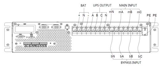
Fig. 2-13 3-phase in and 3-phase out, dual input
