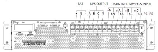
Fig. 2-12 3 phases in 3 phases out, common input
