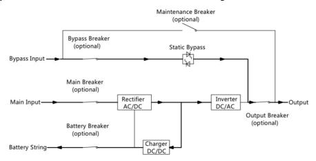
Figure 1-8 ECO Mode operation diagram
