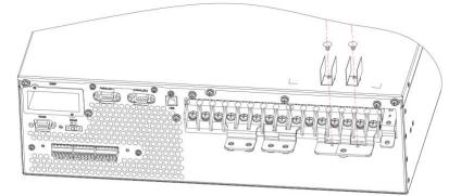
Fig. 2-20 Fix insulation film
