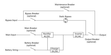
Figure 1-3 UPS Block Diagram
