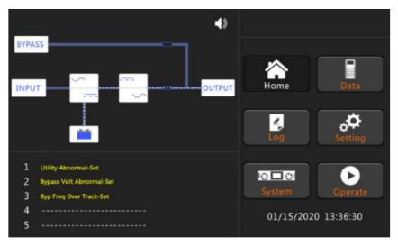
Figure 4-8 Energy flowing diagram of the start completed from batteries 4) Close the external output power supply isolators to supply the loads, and the system is working in battery mode.
