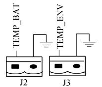
Figure 2-11 J2 and J3 for temperature detecting
