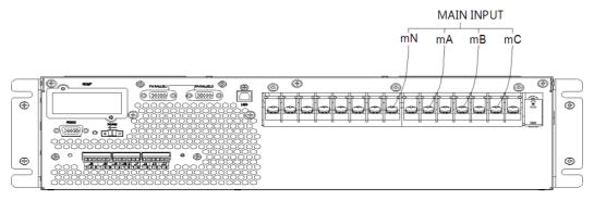
Fig. 2-14 Main line input connection diagram
