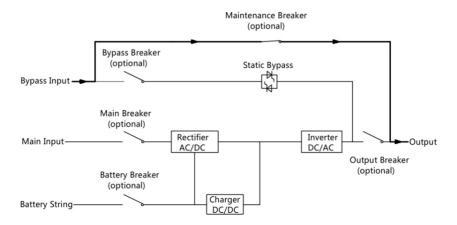
Figure 1-7 Maintenance mode operation diagram
