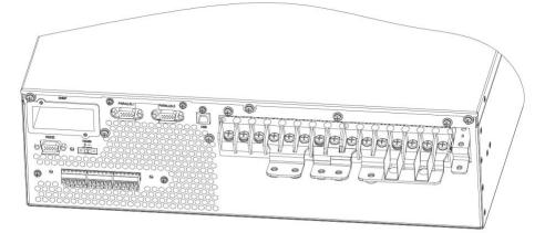
Fig. 2-18 Graphic of insulation film fixed
