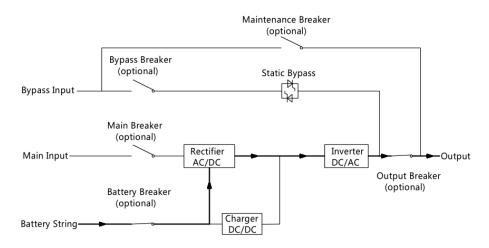
Figure 1-5 Battery Mode operation diagram
