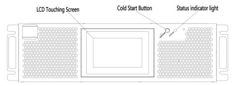
Figure 4-6 Position of the battery cold start button
