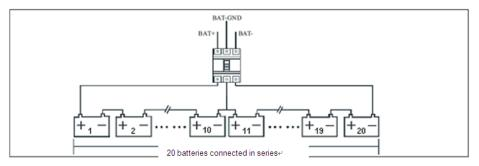
Figure 2-4 Battery connection diagram
