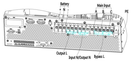
Fig. 2-19 3-phase in and 1 phase out, dual input
