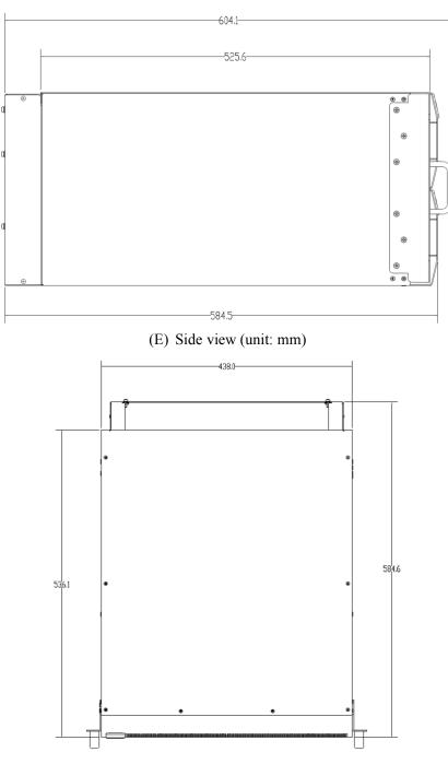
(F) Top view (unit: mm) Figure 2 POD for parallel system outlook
